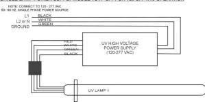
3)ENSURE THE MAIN POWER TO THE AIR HANDLER IS TURNED OFF BEFORE PROCEEDING. Refer to the electrical diagram for proper connection of the power supply to the low voltage power source. CONNECT IN ACCORDANCE WITH ALL STATE AND LOCAL ELECTRICAL AND BUILDING CODES.
