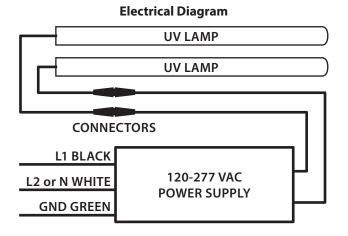
IMPORTANT! Connect in accordance with all state and local electrical and building codes. Proper voltage is automatically selected by the unit between 120–277 VAC Single Phase 50/60 hz. IMPORTANT! An external power suppressor is suggested if power surges occur often.
