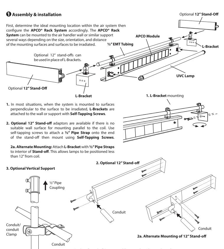
**3. Optional Vertical Support** adds strength to the conduit tubing support framework and prevents sagging on installations with two or more lamps per tubing length. Measure the distance from floor to ceiling then measure and cut tubing 1.75" less than that length. Use the ½" Pipe Couplings to extend the Vertical Support to floor and ceiling for a snug fit.
