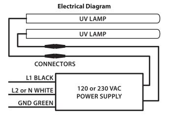
IMPORTANT! Connect in accordance with all state and local electrical and building codes. Proper voltage is automatically selected by the unit between 120 or 230 VAC Single Phase 50/60 hz. IMPORTANT! External power suppressor may be needed if power surges occur.
